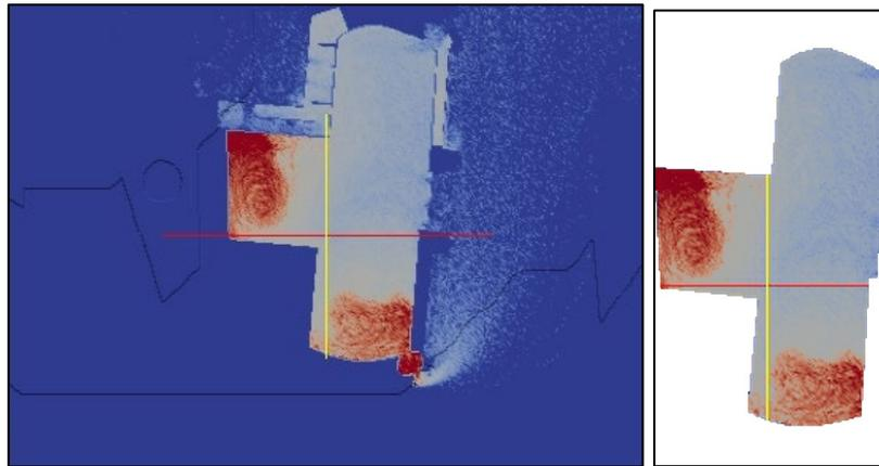
**Figure 4**, Ground concentration computed in the Grand Palais nested domain (left hand side) and close-up view of the largest room (right hand side). Concentrations are ranging from low values (blue) to large values (red)
